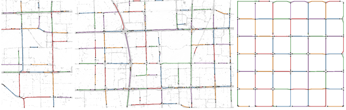
Figure 5: Extracted junction graphs. (work in progress) The first two are computed on 500 trajectories from the Beijing taxi data set, the third one on synthesized trajectories on a grid network.
