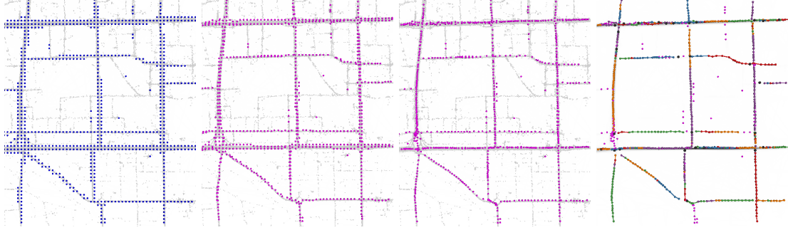
Figure 3: Example of the first iteration in the skeleton extraction process. Figure 1-3 illustrates the contraction of skeleton points to the road centerline. In the left most figure, blue points show the initial location of the skeleton points, sampled uniformly from the voting image; The middle two images are two intermediate steps of the contraction. The right most figure draws the branches traced after the contraction stops.
