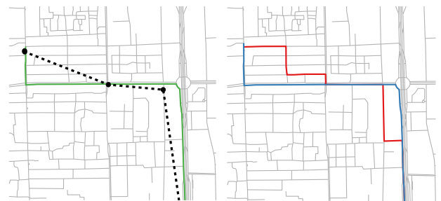
Figure 1: Left: A sparse trajectory (black) and its ground truth path (green); Right: Projected paths of the trajectory in the left figure using data-driven map matching (blue) and single-track map matching (red).
