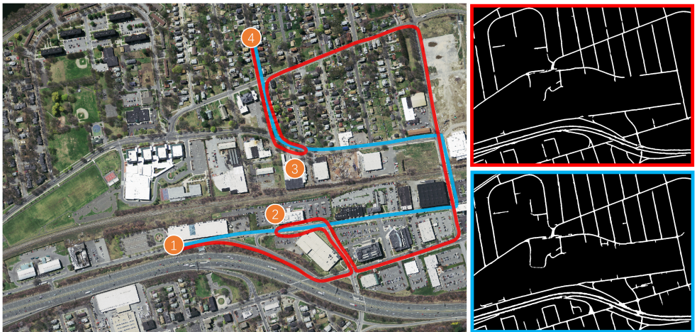
Figure 1: Significance of topological accuracy in road segmentation and subsequent route planning. The figure contains an aerial image from Massachusetts alongside two segmented road maps predicted by U-Net (top) [40] and ours (bottom), respectively. These two segmentation results achieve similar quality in per-pixel accuracy, but the top one is observed to have more broken roads. Road graphs are extracted from these segmentation [6] and further generate different optimal paths to visit the four locations in the image, which are depicted in red and blue, respectively. Bottom segmentation is evidently preferred, because the blue path is much shorter than the red one.
