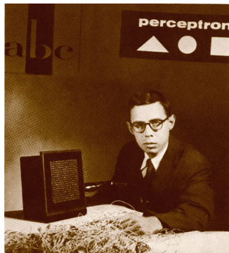
Hardware implementation: Mark I Perceptron
